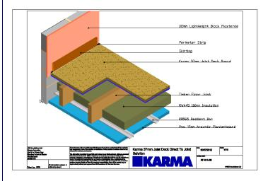
**Application:** Easy to fit, slimline solution for existing timber joist floors where the original floorboards need to be replaced. The new or existing ceiling below is decoupled. Can also be used as a solution if there is no access to the ceiling below.
